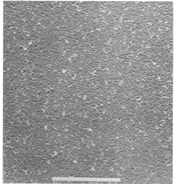
Figure 3 Electron micrograph of fully developed ultra-low expansion transparent glass-ceramic of composition 1 (white bar = 1 μm).
