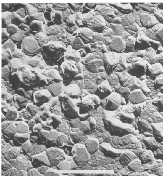
Figure 5 Electron micrograph of fully developed refractory and transparent glass-ceramic of composition 2. (white bar = 1 \mu\text{m} )
